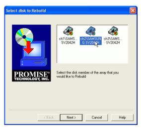
Figure 77. Rebuild Wizard disk drive selection window.
